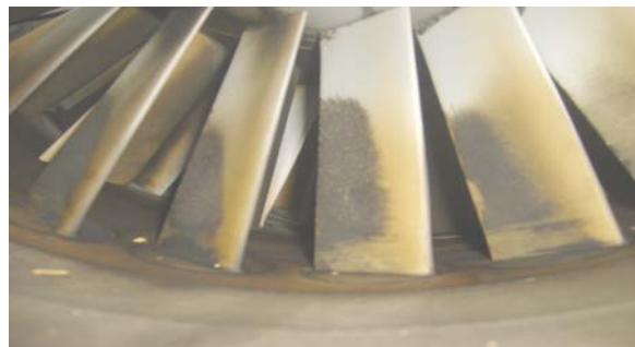
Figure 1: Compressor fouling on first stage (Inner Guide Vane (IGV) after 8000 firing hours.)
