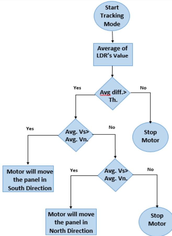
Figure 4: Flow chart of the algorithm used by Arduino.
