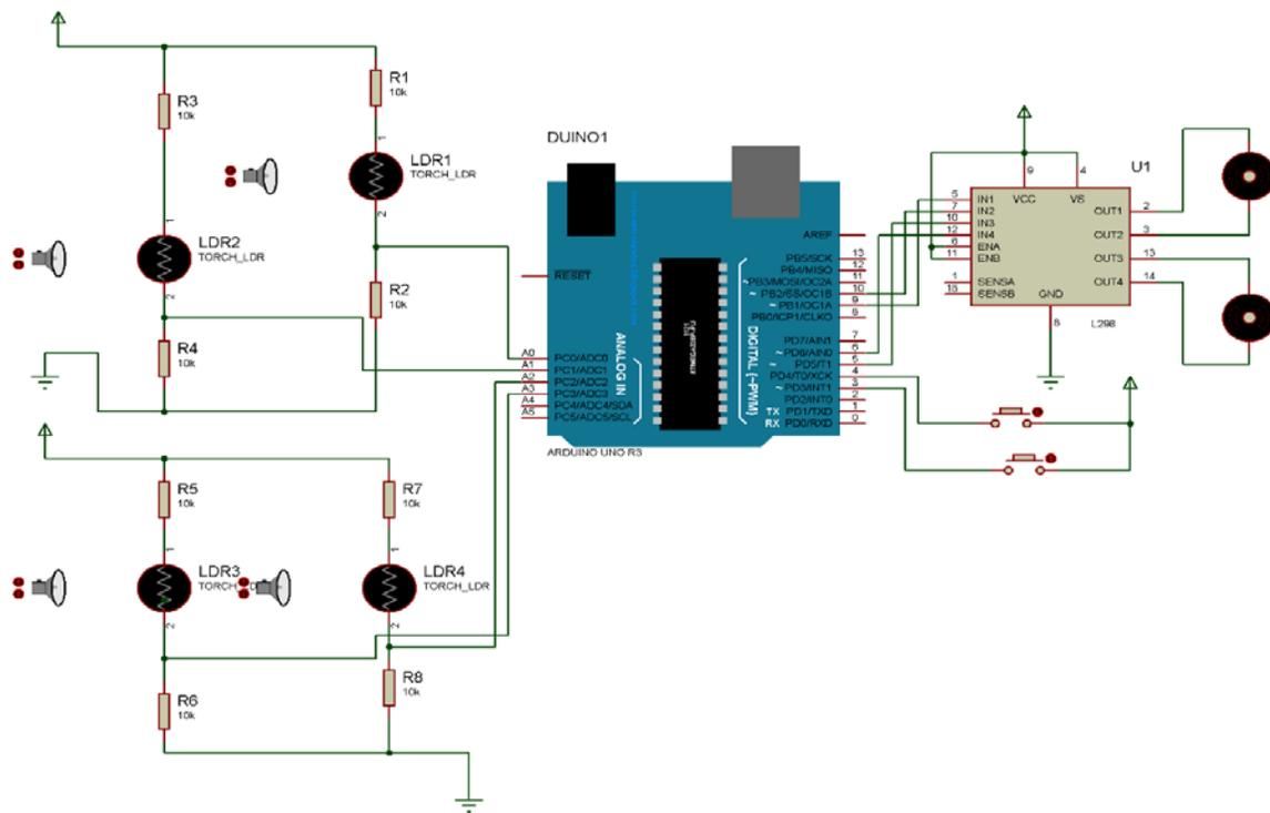
Figure 3 (b): Circuit diagram of solar tracking system.
