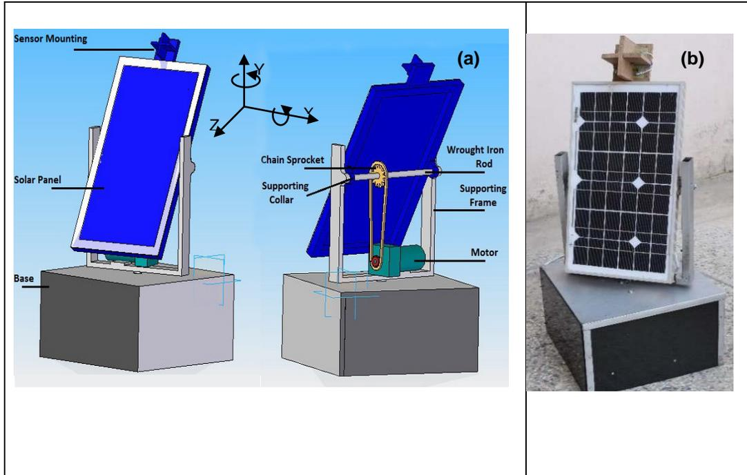
Figure 1: (a) Model of solar tracking system, (b) Solar tracking system.
