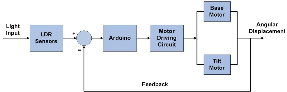
Figure 3 (a): Block Diagram of the solar tracking system.
