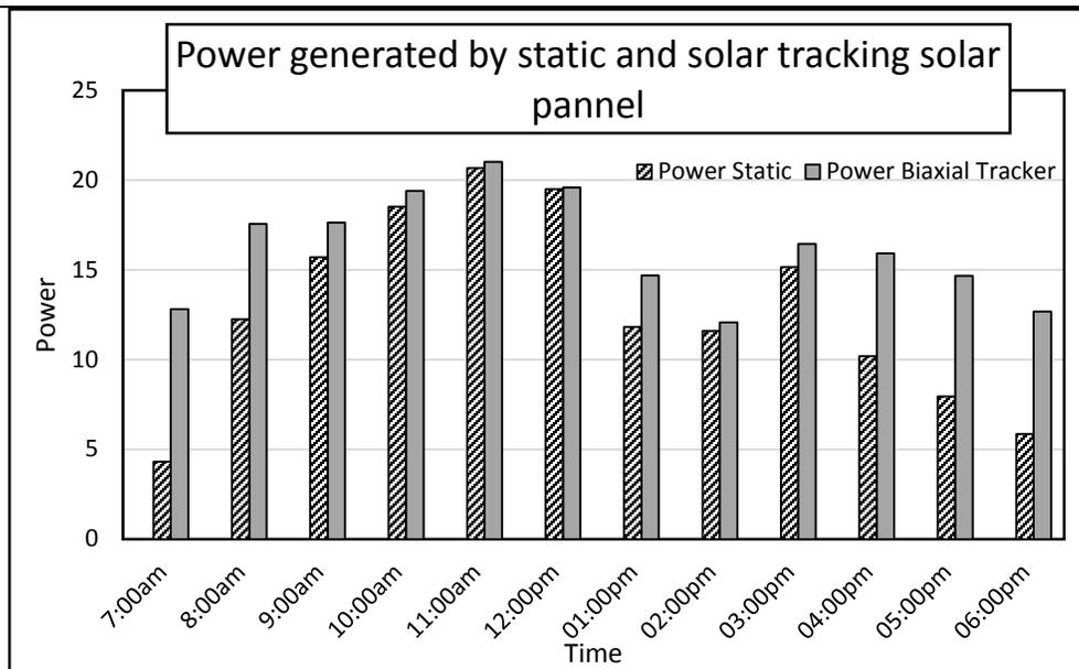
**Figure 5: Comparison of power output for static and biaxial solar panel**
