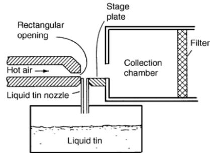
Figure 1: Cross – jet gas atomization scheme. [3]
