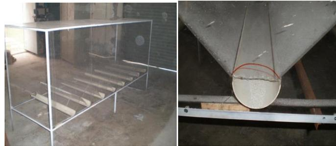
Figure 3: A view of the atomizing chamber and tin metal powder in one partition of collection slot in the chamber.
