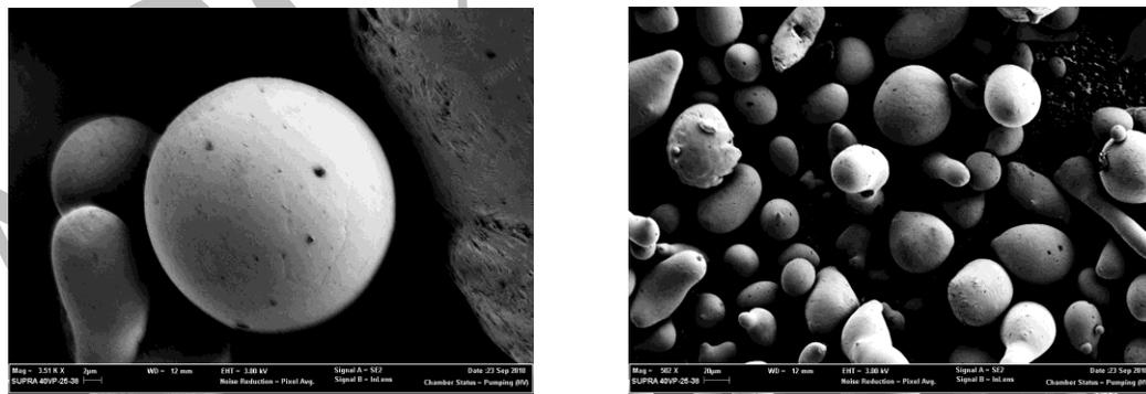
Figure 4: Scanning electron micrographs of gas atomized tin powder.
