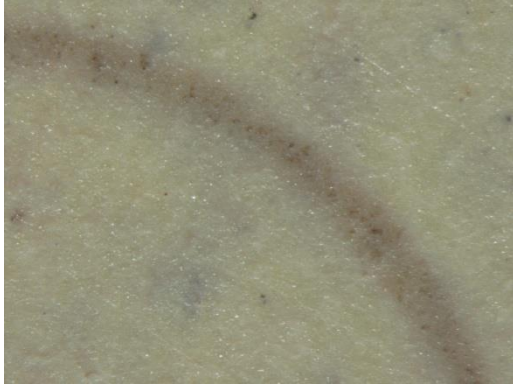
Fig.5 Wear track of coating on MS at 6N load at room temperature
