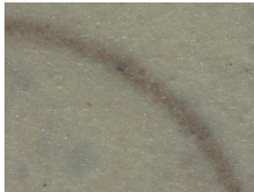
Fig.2 Wear track of coating on SS at 2N load at room temperature
