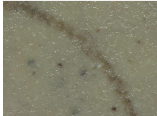
Fig.8 Wear track of coating on MS at 6N load at 100°C
