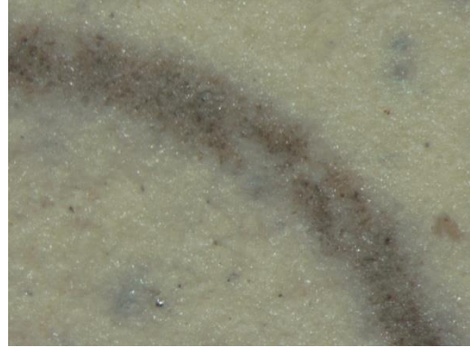
Fig.6 Wear track of coating on MS at 6N load at room temperature
