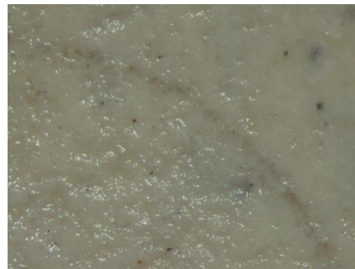
Fig.4 Wear track of coating on SS at 2N load at 100°C
