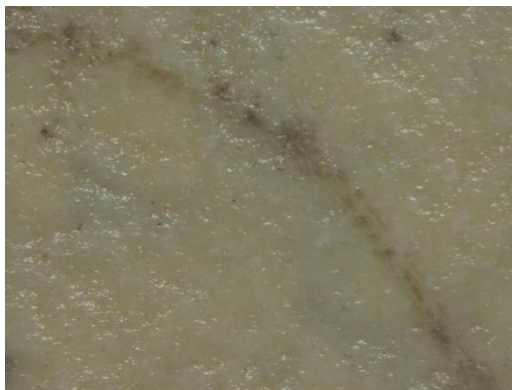
Fig.3 Wear track of coating on MS at 2N load at 100°C
