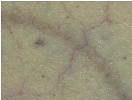
Fig.1 Wear track of coating on MS at 2N load at room temperature
