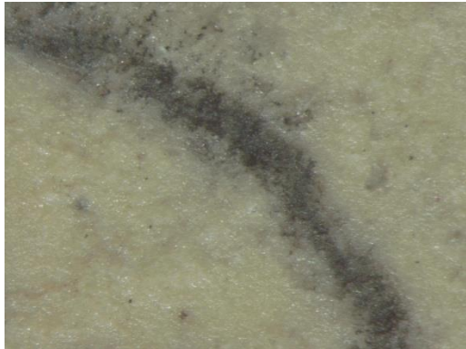
Fig.7 Wear track of coating on MS at 6N load at 100°C
