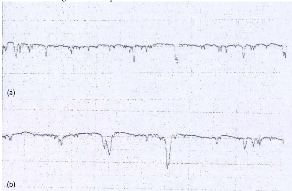
Fig. 7 Surface profile of wear tracks at 8N load and temperature of (a) 50°C and (b) 100°C.
