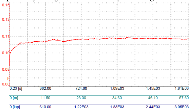
Fig. 4 Friction co-efficient with varying time, sliding distance and no. of laps at 50°C and 8N load.
