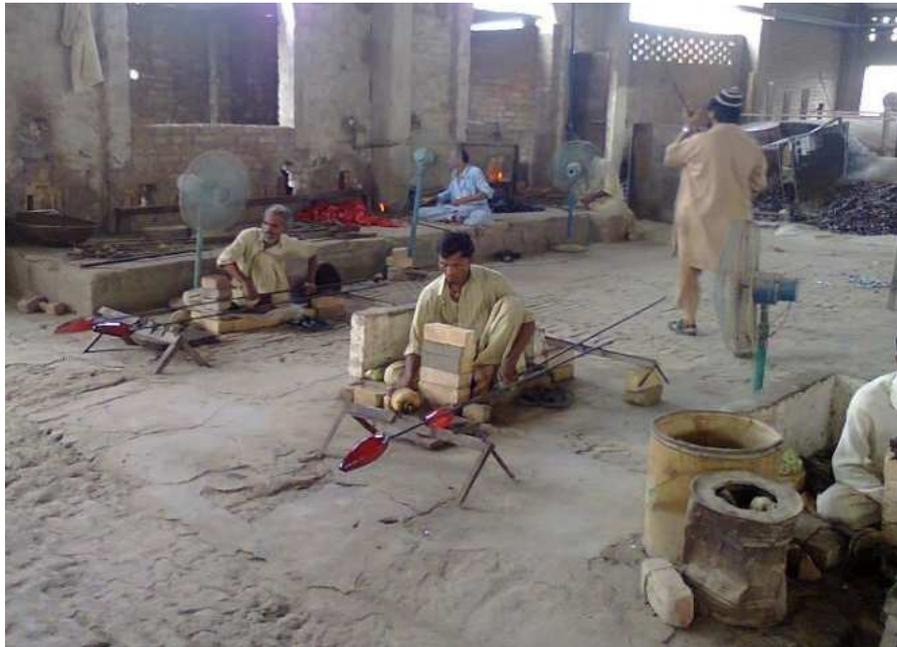
**Figure 3: Gob prepared by manually gathering different coloured molten glasses on gathering rod is ready to be drawn into spiral form bangles.**
