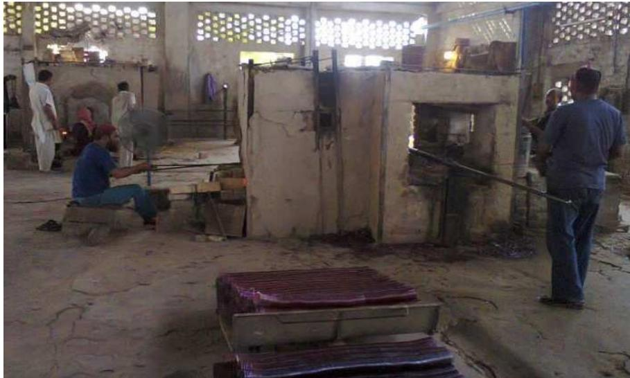
**Figure 4: Manually gathered gob on gathering rod is being formed into bangle at Shadman Glass Works, Hyderabad.**
