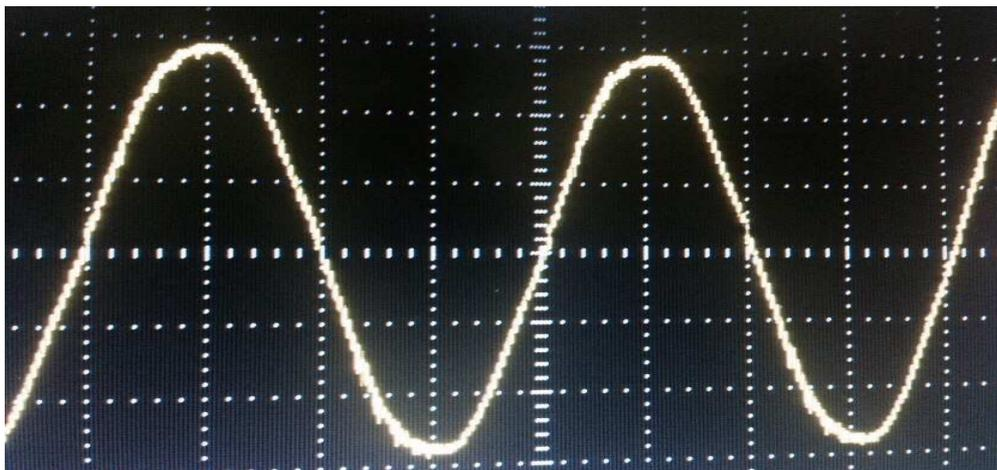
**Figure 6: Synchronized output wave form**
