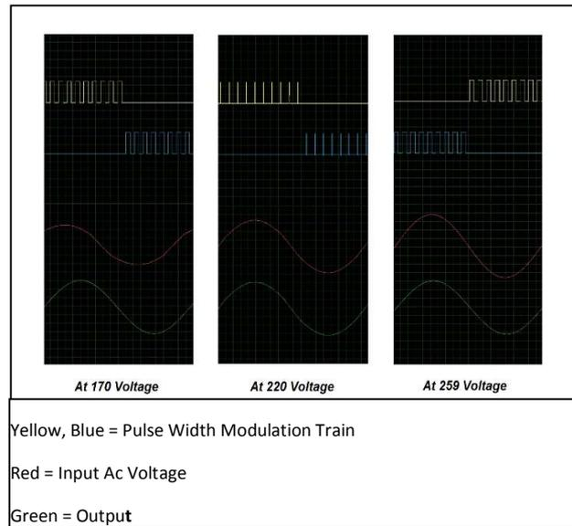
Pulses that are produced from the microcontroller according to the input, are then fed to a current booster circuit, where these pulses are amplified enough to drive the IGBTs [10].
