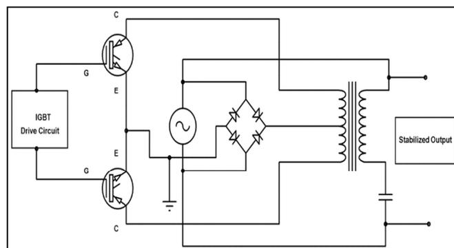
**Figure 4: Buck/Boost Section of Stabilizer**
