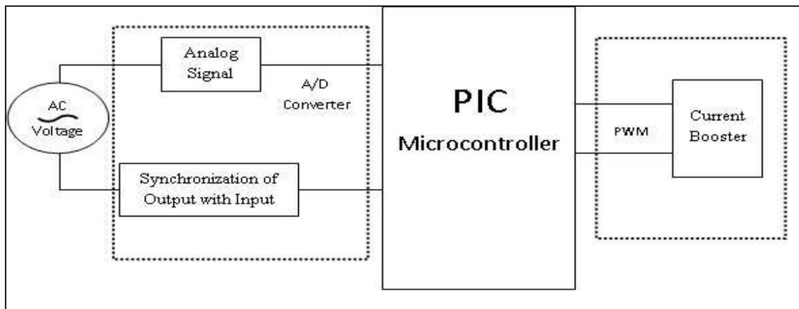
**Figure 2: Control Section of Stabilizer**
