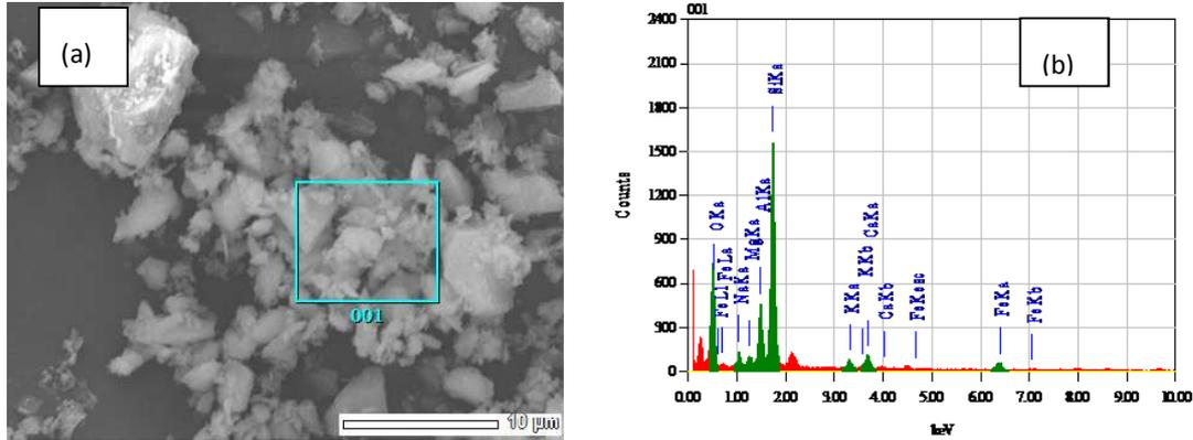
Figure 3. (a) FESEM, (b) EDX analysis of silica sand nanoparticles.
