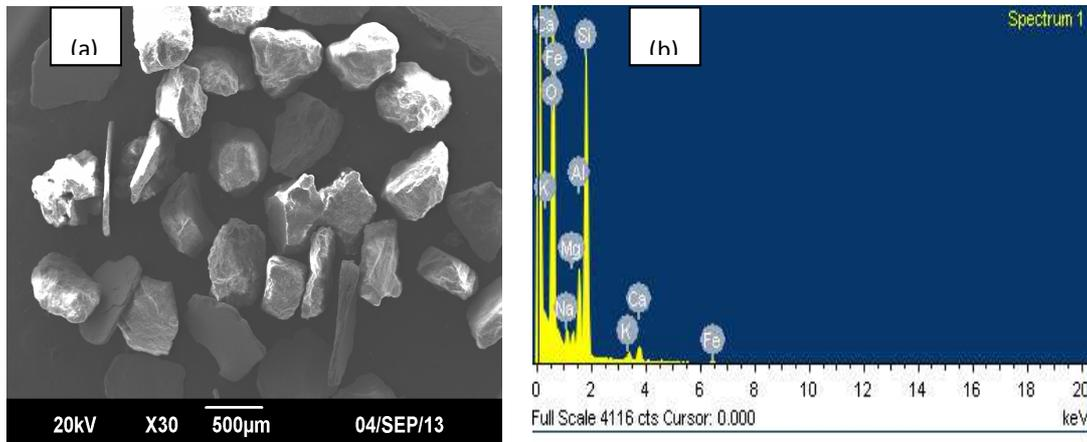
Figure 1. (a) FESEM, (b) EDX analysis of Thal Silica Sand.
