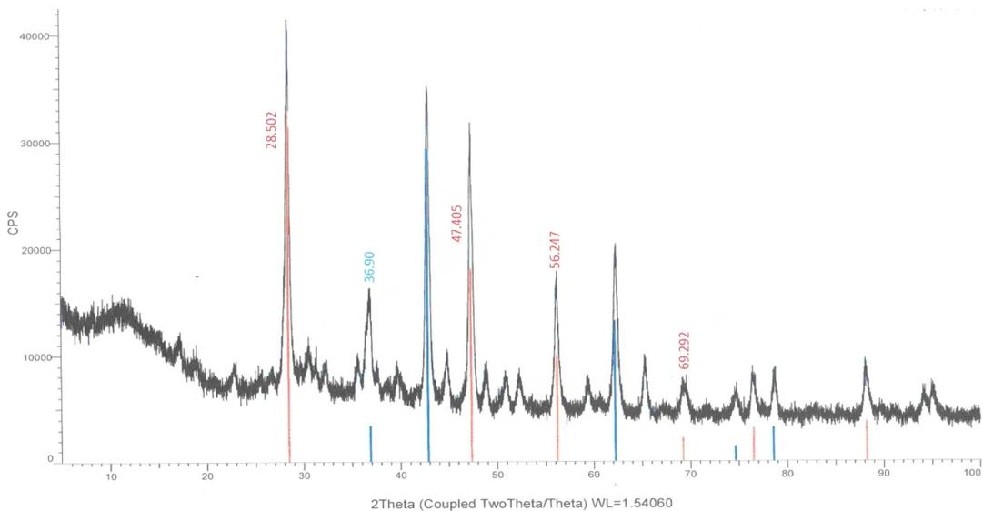
**Figure 6. XRD analysis of silica sand under Argon at 900°C.**
