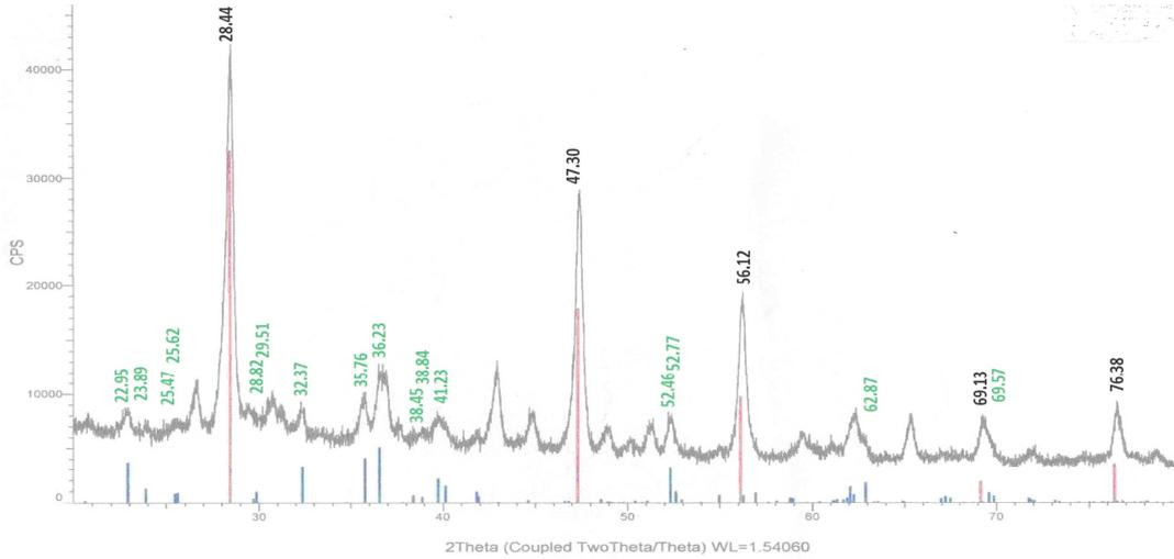
**Figure 5. XRD analysis of silica sand without Argon at 900°C.**
