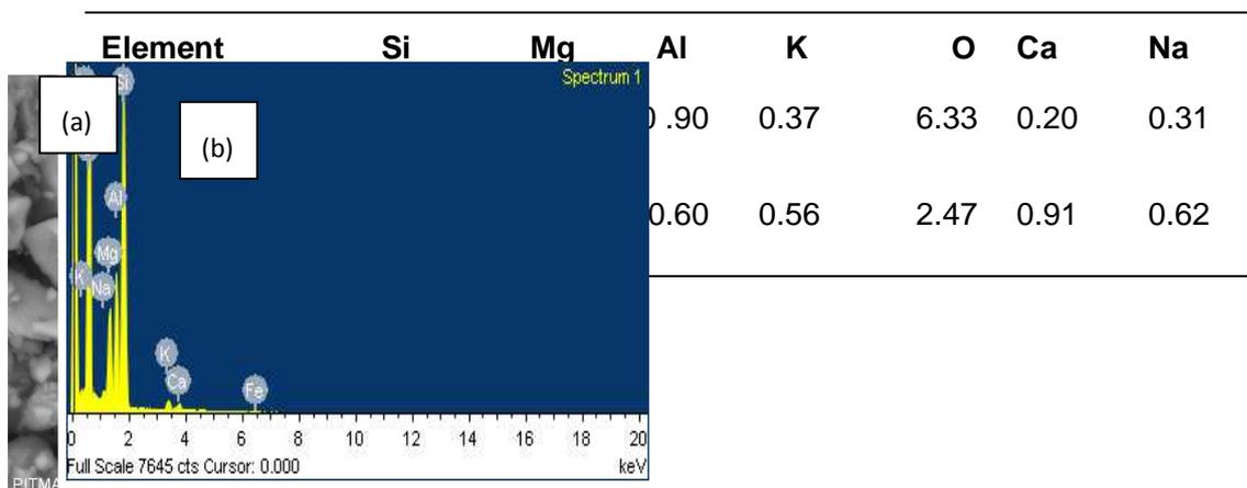
**Figure 7. (a) FESEM, (b) EDX analysis of leached silicon powder.**
