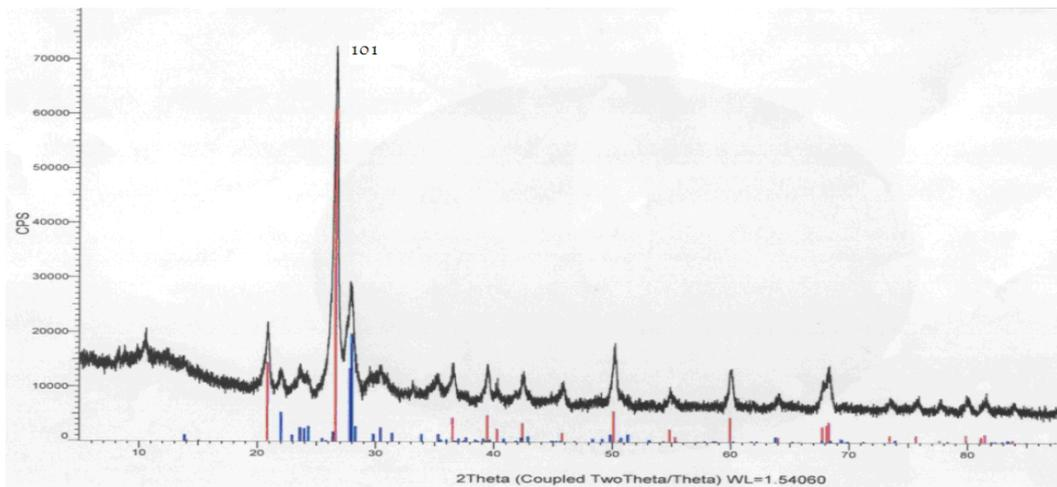
**Figure 4. XRD Analysis of the Thal Silica Sand.**
