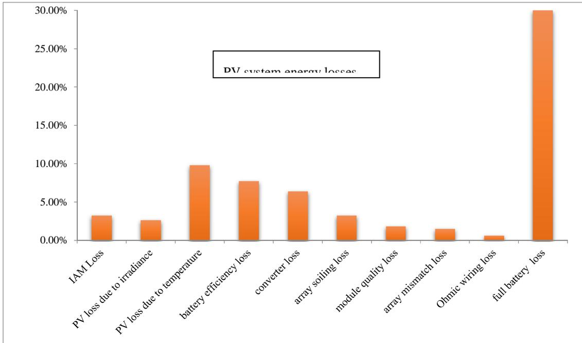
**Figure 3: PV system energy losses**
