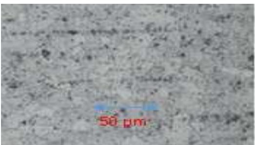
Figure 14. HAZ of AA6061 Aluminum Alloy.
