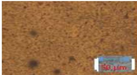
**Figure 2. HAZ of AA6061 Aluminum Alloy.**
