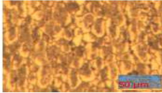
**Figure 6. TMAZ of AA2024 Aluminum Alloy.**
