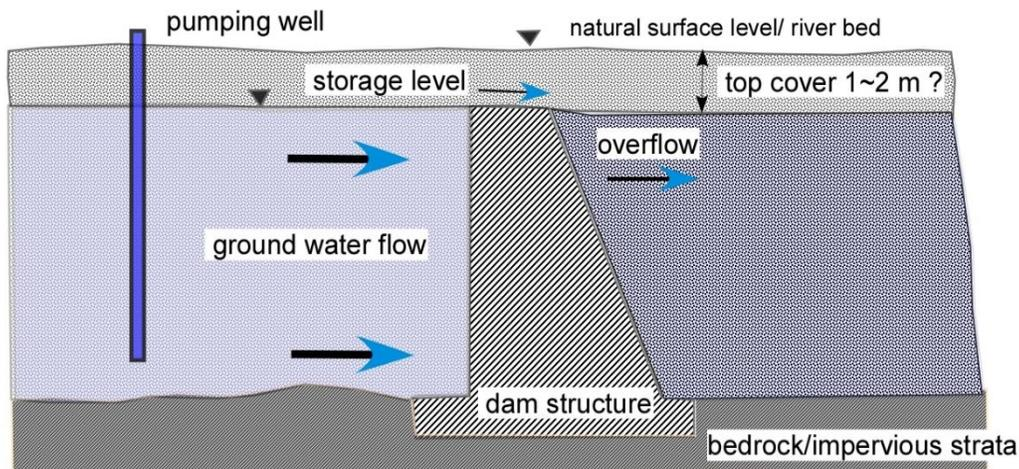
Figure 1. Typical scenario for a subsurface dam
