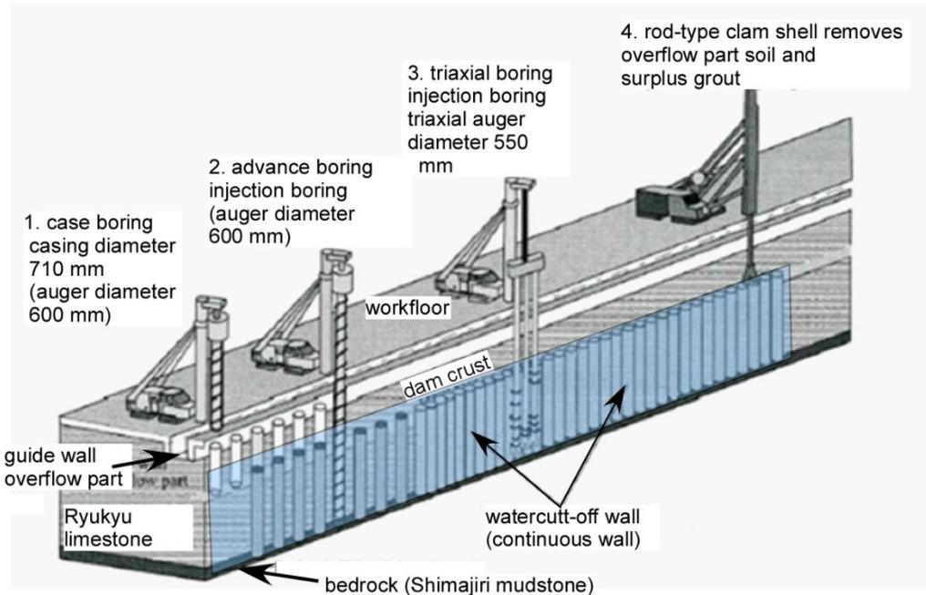
**Figure 4. Conceptual diagram of the mix-in-place (or soil mixing) construction method (modified after [5]).**
