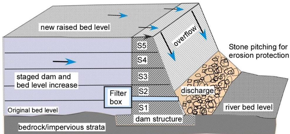
**Figure 2. Schematic representation of a staged sand storage dam**
