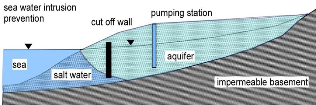
**Figure 3. Typical cross section illustrating how a cutoff wall can serve as a saltwater intrusion prevention dam (modified after [5]).**
