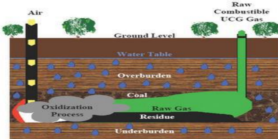
Figure 4. UCG Production Process
