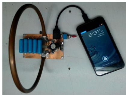
Figure 12. A snapshot of charging of a cell phone using Wireless Energy Transfer System
