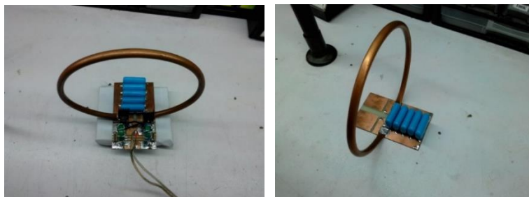
Figure. 3 Snapshot of Resonant coils of Wireless Energy Transfer System (a) transmitter (b) receiver
