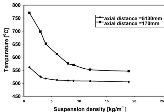
**Fig 4:** Variation of temperature between bottom and top of the riser with suspension density [ $U=4.5$  m/s,  $T_b=600^{\circ}\text{C}$ ]
