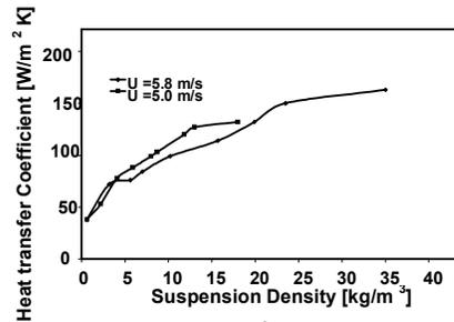
**Fig.11:** Effect of Suspension density on heat transfer coefficient [T<sub>b</sub> = 750 °C]
