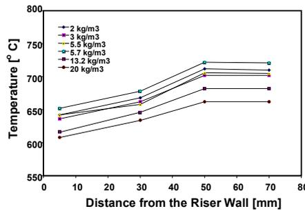
Fig. 5: Radial Temperature Profile in the Riser [ $T_b = 720^{\circ}\text{C}$ ,  $U=5.0\text{ m/s}$ ]
