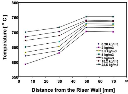
**Fig. 7:** Radial temperature profile in the riser [T<sub>b</sub> = 800 °C, U = 5.6 m/s]
