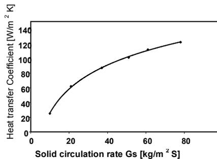
**Fig.14:** Effect of solid circulation rate on heat transfer coefficient
