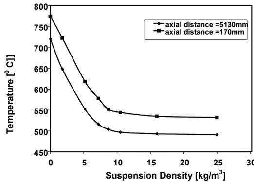
**Fig 3:** Variation of temperature between bottom and top of the riser with suspension density [ $U=5$  m/s,  $T_b=750^{\circ}\text{C}$ ]
