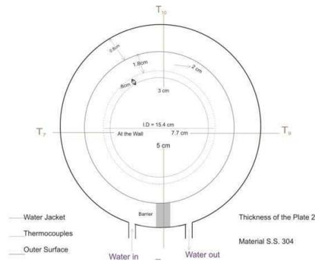
**Figure 2:** (a) Schematic of cooling plate for radial heat transfer studies [with thermocouples and accessories]
