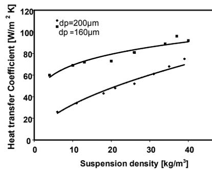
Fig.13: Effect of suspension density on heat transfer coefficient
