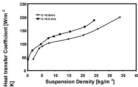
**Fig.10:** Effect of Superficial gas Velocity on heat transfer coefficient [T<sub>b</sub> = 700 °C]
