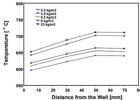
Fig. 6: Radial Temperature Profile in the Riser [ $T_b = 775^{\circ}\text{C}$ ,  $U = 5\text{ m/s}$ ]
