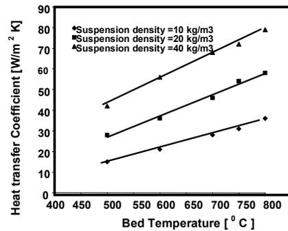
Fig.12: Effect of bed temperature on heat transfer coefficient
