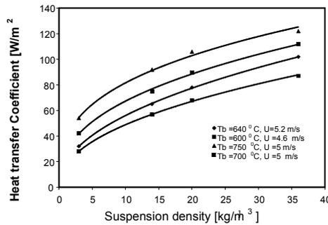
**Fig 9:** Effect of suspension density on heat transfer coefficient
