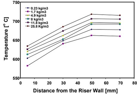
**Fig. 8:** Radial temperature profile in the riser [T<sub>b</sub> = 820 °C, U = 5.8 m/s]
