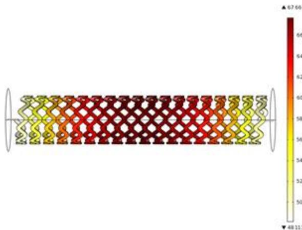
Figure 10: Temperature distribution along the stent surface at 3V of applied voltage, simulation result
