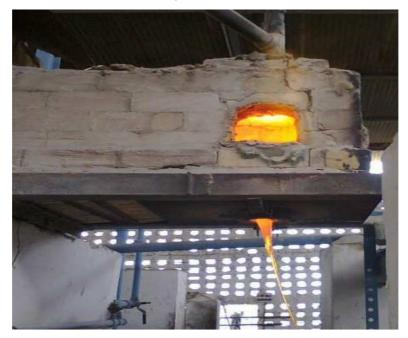
Figure 1: Molten glass coming out of the single gob orifice ring in the form of continuous thread.
