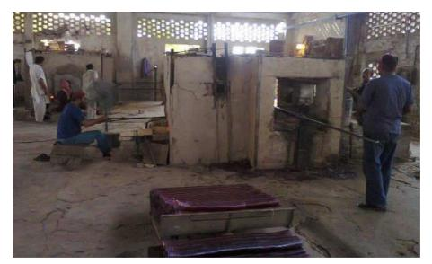
Figure 4: Mannually gathered gob on gathering rod is being formed into bangle at Shadman Glass Works, Hyderabad.
