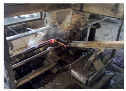
Figure 2: Continuous thread of hot glass rotating onto a roller forming into spiral shaped bangle.
