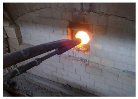
Figure 5: Gas fired burner being used in glass melting furnace.
