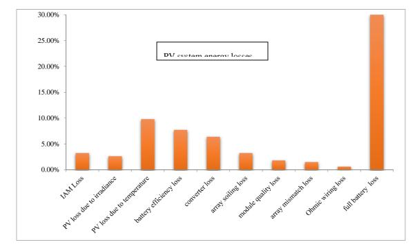
Figure 3: PV system energy losses
