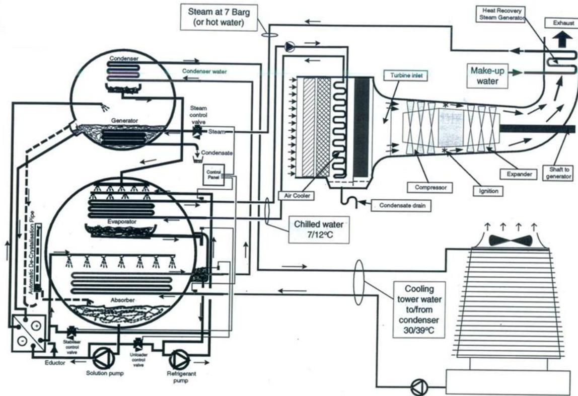
Figure 2. Inlet air cooling system
