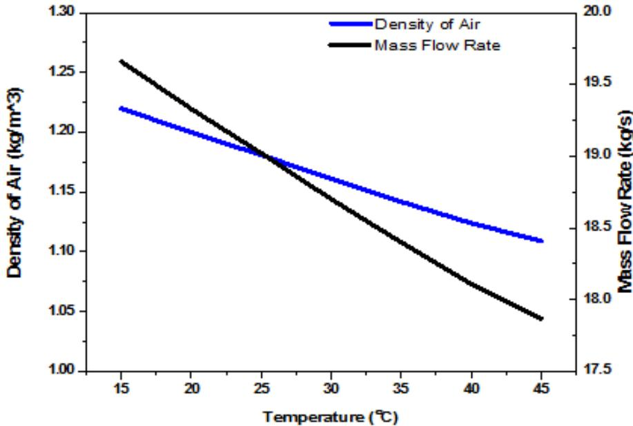
Figure 3. Graph between Density, Mass Flow Rate of Air and Temperature
