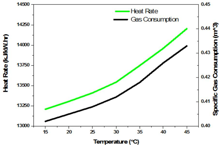
Figure 5. Graph between Heat Rate, Specific Gas Consumption and Temperature
