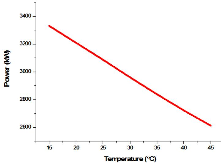
Figure 4. Graph between the Power Output of the Gas turbine and Temperature
