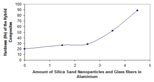
Figure 4. Hardness (HV) of Aluminium based Hybrid Composites
