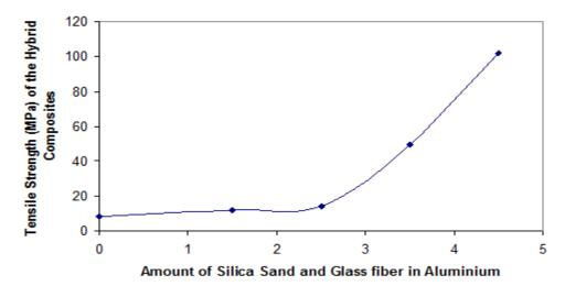
Figure 1. Tensile Strength of the Aluminium based Hybrid Composites
