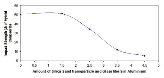
Figure 3. Impact Strength of Aluminium based Hybrid Composites
