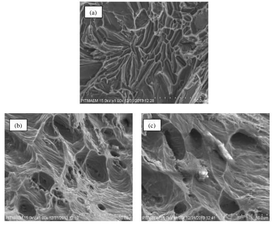
Figure 5 (a, b, c). Fractured Tensile specimen of Aluminium based Hybrid Composites
