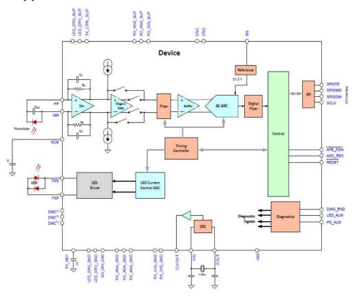
Figure 4. Detailed block diagram for the AFE449 [6]
