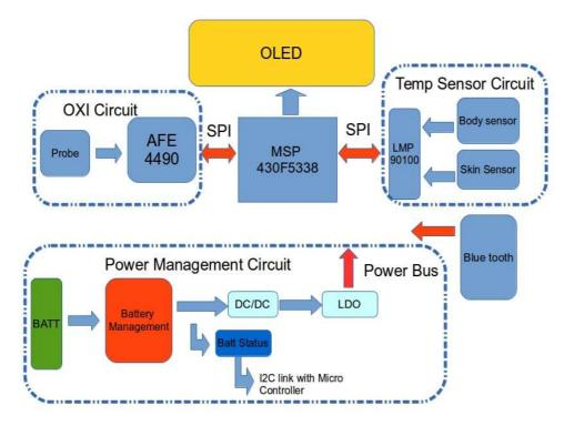
Figure 2. Pulse Oximeter Block Diagram
