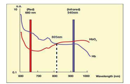
Figure 2. Oxygen bounded versus unbounded blood light absorption of IR and RED lights [3]
