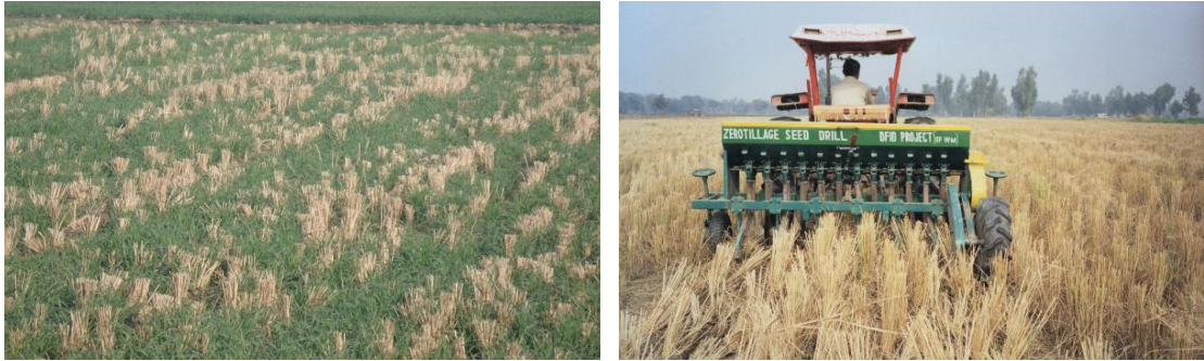
Fig. 3: Paddy stubbles and tractor drawn seed drill sowing wheat in paddy stubbles with zero tillage.
