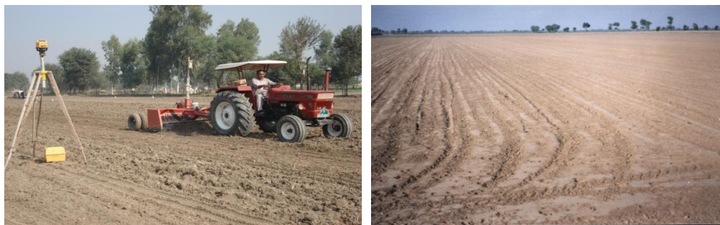
Fig. 2: Laser land leveller in operation and the filed levelled afterwards.
