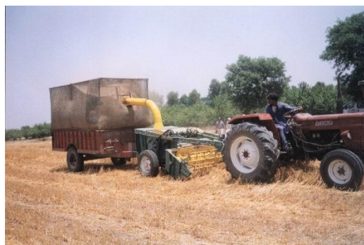
Fig. 8: Wheat straw chopper cutting the wheat stubble in the field.
