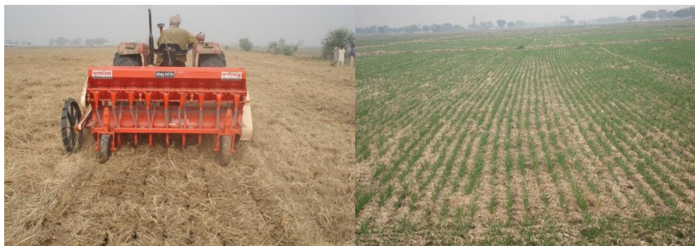
Fig. 7: Combo happy seeder/turbo seeder sowing wheat in crop residues.
