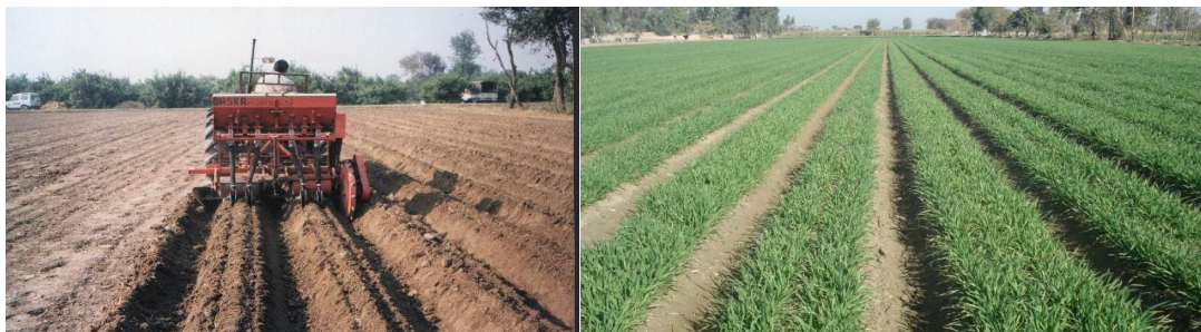
Fig. 6: Bed Planter making beds for wheat sowing and wheat beds afterwards.
