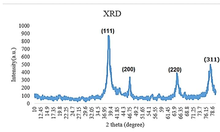
**Fig. 3:** X-ray diffraction pattern of synthesized silver nanoparticles using a combined of *Urtica dioica* and *Scrophularia striata*.
