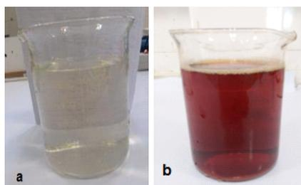
**Fig. 1:** The process of reducing  $Ag^+$  to AgNPs. (a) Color change before reduction and (b) After reduction.
