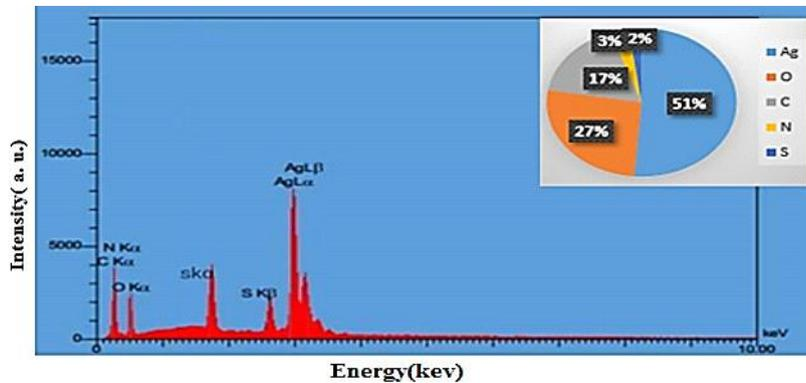
**Fig. 6:** EDX form of biosynthesized silver nanoparticles using a combined extract of *Urtica dioica* and *Scrophularia striata*.
