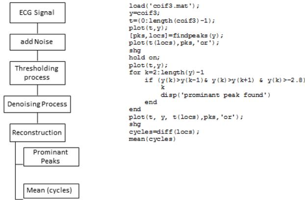
FIGURE 2. Flowchart and Program for Peak Detection
